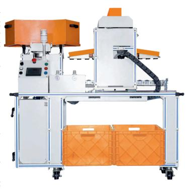
productivity even as it reduces dependability on human resources. The machine comprises of an empty cops insertion chute device, a full cops doffing grippers assembly, a travelling trolley device with an electronic control panel—and can transform your production line.
