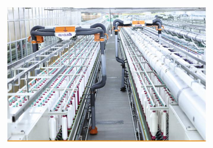
**LPT GLI-CLEAN Belt Drive Model** has a light-weight chamber as the fan motor is designed to be stationary at the track end. The light-weight chamber delivers superior efficiency including:• Higher blowing and suction performance.
