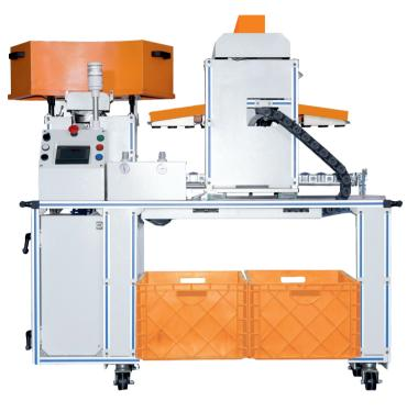
alternative. **DYNADOFF** adds value by increasing productivity even as it reduces dependability on human resources. The machine comprises of an empty cops insertion chute device, a full cops doffing grippers assembly, a travelling trolley device with an electronic control panel—and can transform your production line.
