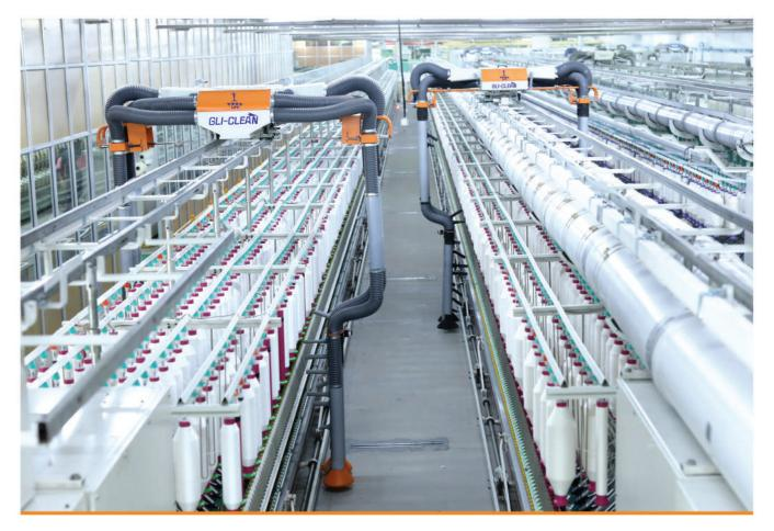
**LPT GLI-CLEAN Belt Drive Model** has a light-weight chamber as the fan motor is designed to be stationary at the track end. The light-weight chamber delivers superior efficiency including: • Higher blowing and suction performance.
